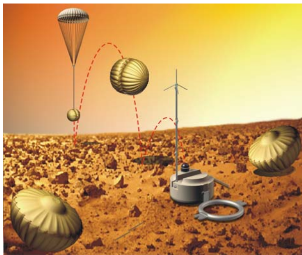
Figure 7: Final steps in the EDL phase: - First contact with the ground (Touchdown) - Several rebounds - Pyrotechnic separation of the airbags - Upright orientation manoeuvre of the Mars station
